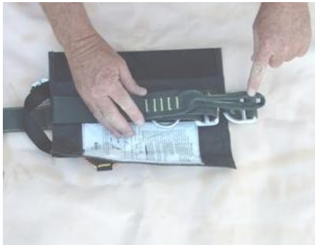
Step 3: The strap is folded with the Shane ring protruding from the front of the pouch.
