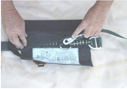
Step 1: Open the pouch and lay the strap front to back, pouch notice the buckle (Dutchmen).
