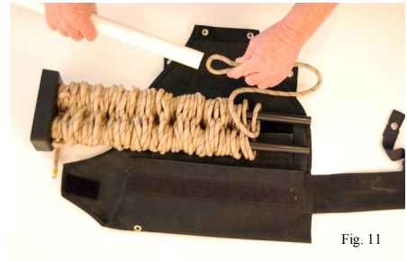
Create a bite at end of rope and insert into outer tube.
