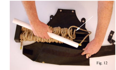
IMPORTANT: To ensure deploys properly, the first loop must feed from top inner tube shown by arrow. Feed outer tube thru sleeve.
