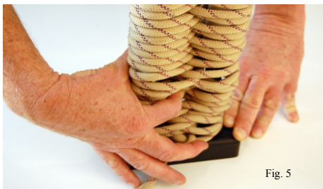
Use your index finger and thumb to alternately displace the rope coils to the level of the outer tubes.
