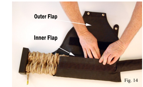
Place rope and jig in bag and lightly Velcro the inner flap.
